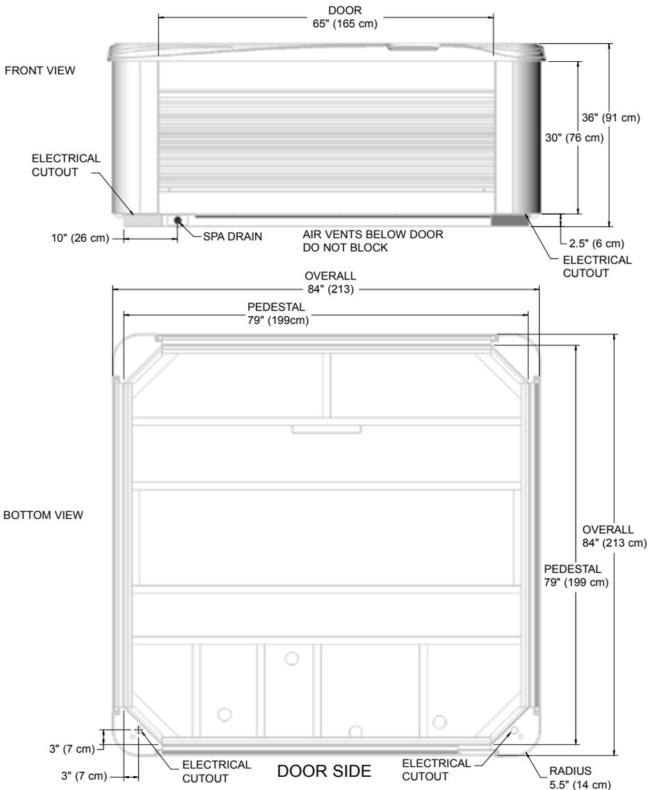
**NOTE: WATKINS WELLNESS** recommends that the **REUNION** be installed on a minimum 4" (10 cm) thick reinforced concrete pad or structurally sound deck able to support the "dead weight" found in the chart on the back page.
