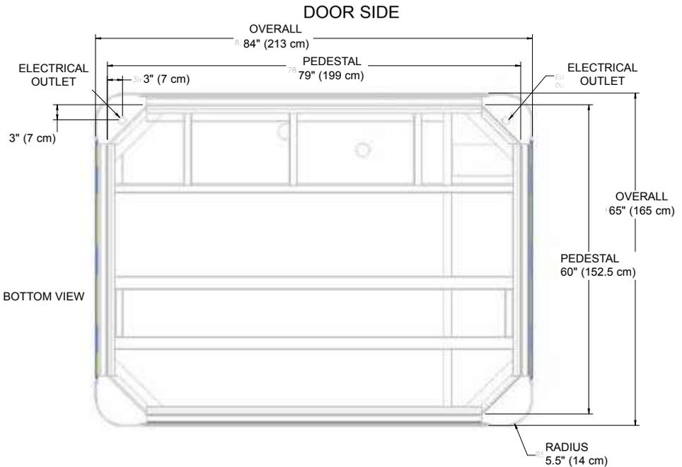
**NOTE: WATKINS WELLNESS** recommends that the **KAUAI** be installed on a minimum 4" (10 cm) thick reinforced concrete pad or structurally sound deck able to support the "dead weight" found in the chart on the back page.
