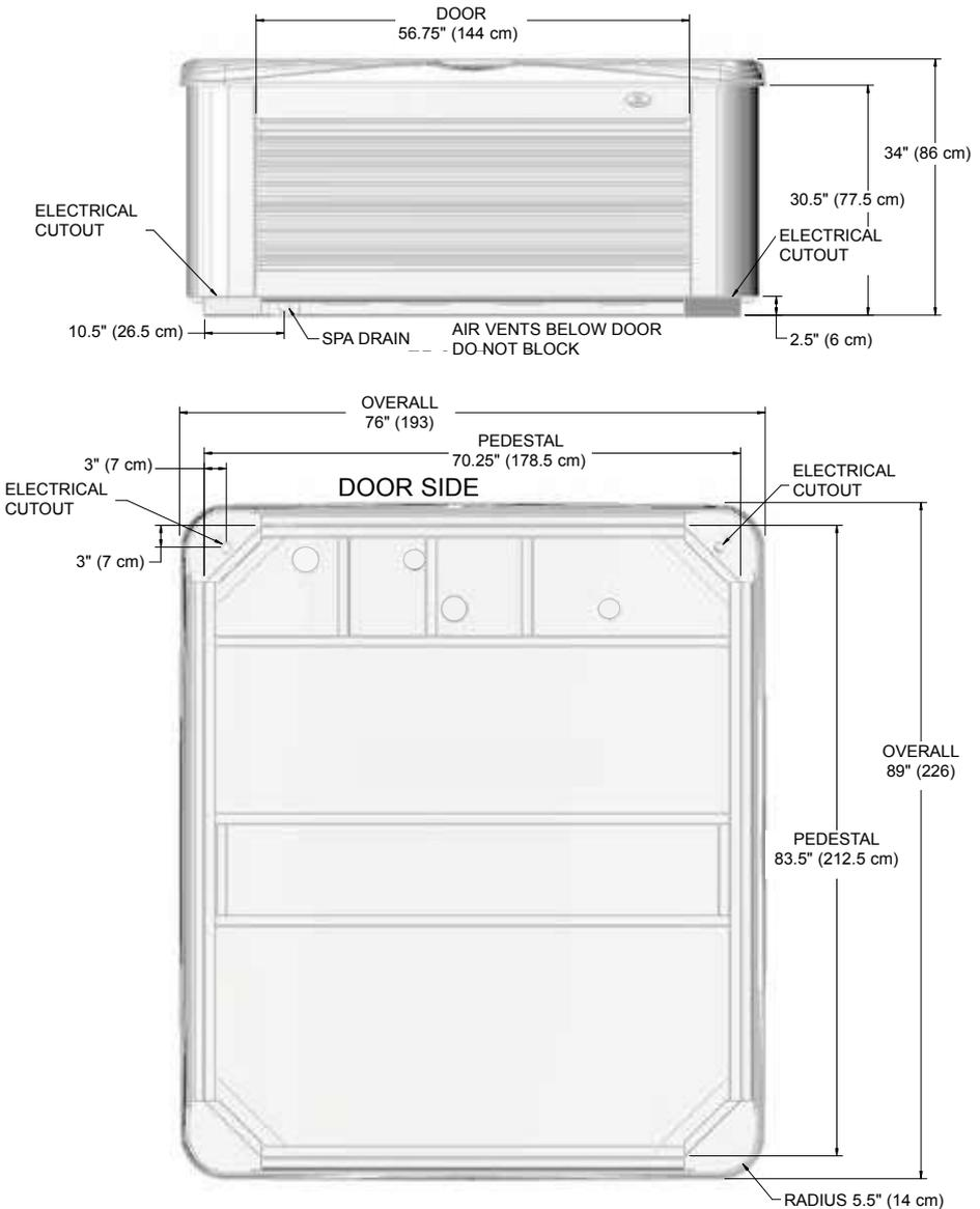
**NOTE:** WATKINS WELLNESS recommends that the **MARTINIQUE** be installed on a minimum 4" (10 cm) thick reinforced concrete pad or structurally sound deck able to support the "dead weight" found in chart on the back page.
